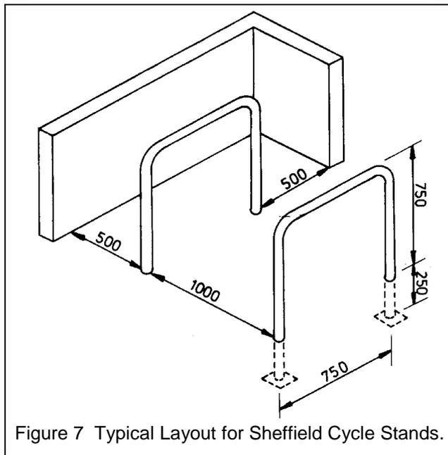
Figure 7 Typical Layout for Sheffield Cycle Stands.
