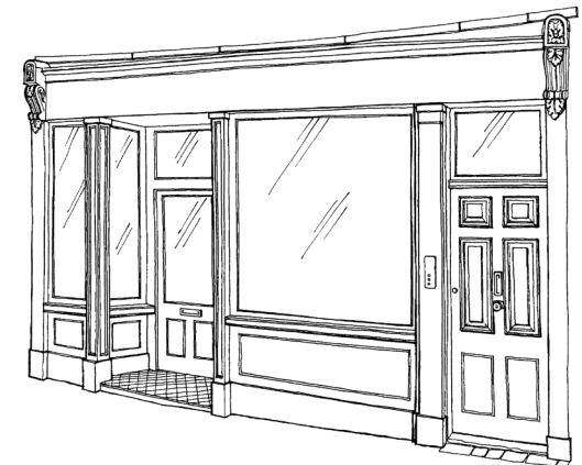
Doors to upper floors should be treated as integral to the design of the shopfront
