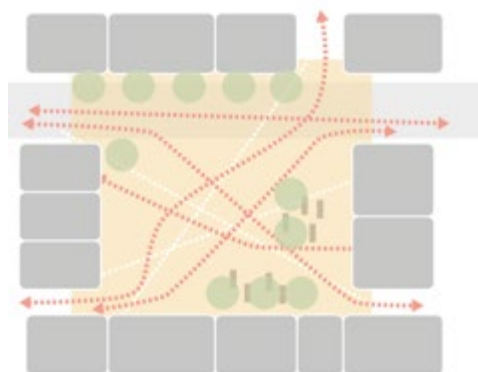
Fig 52 Movement: A study of the needs, orientation and pedestrian movement is important to design a public space.
