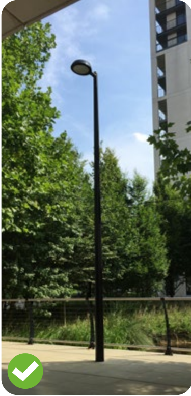
Fig 74 Columns in vehicular areas that are simple, robust, with consistent colours at 5-7m high
